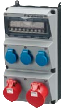
AMAXX® combinations from AMELAN®. High resistance to chemicals, highly heat resistant contact carriers and nickel plated contacts for use in an aggressive atmosphere.
